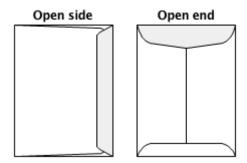
**Flap Styles** The flap is the part of the envelope that is folded to seal the envelope. The main flap shapes are shown in the illustration.
